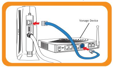
5. Connect one end of the yellow cable to the yellow port labeled "Ethernet 1" on the back of the Vonage Device. Connect the other end to the Ethernet port on your computer or router that you unplugged earlier.
